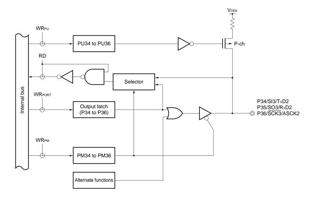
Figure 6-10. P34 to P36 Block Diagram (µPD780078Y Subseries)
