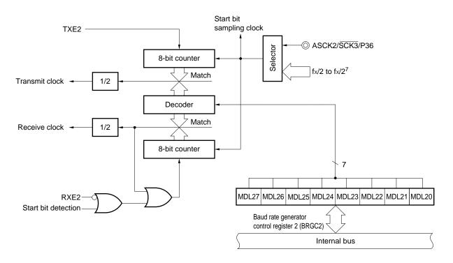
Remark TXE2: Bit 7 of asynchronous serial interface mode register 2 (ASIM2) RXE2: Bit 6 of asynchronous serial interface mode register 2 (ASIM2)
