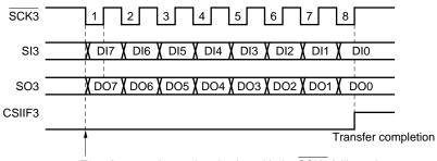
Transfer starts in synchronization with the SCK3 falling edge
