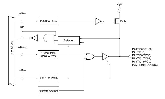
PU : Pull-up resistor option register
