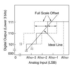
Figure 13-14. Differential Linearity Error
