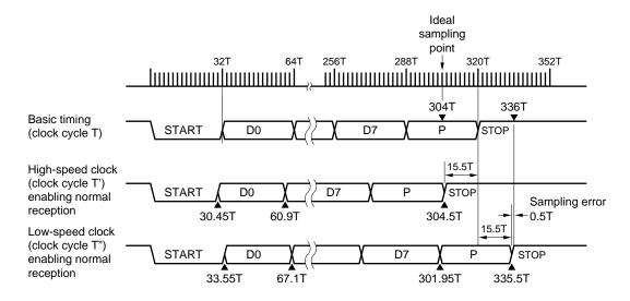
Figure 14-6. Error Tolerance (when k = 0), Including Sampling Errors
