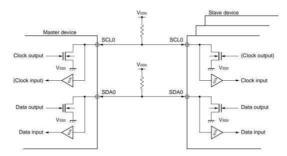
Figure 18-6. Pin Configuration Diagram
