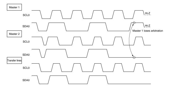
Figure 18-14. Arbitration Timing Example
