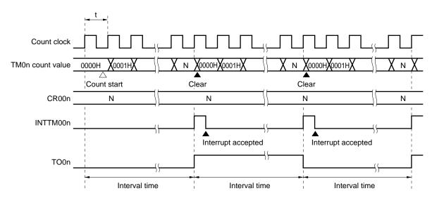
**Remark** Interval time =  $(N + 1) \times t$ N = 0000H to FFFFH n = 0, 1
