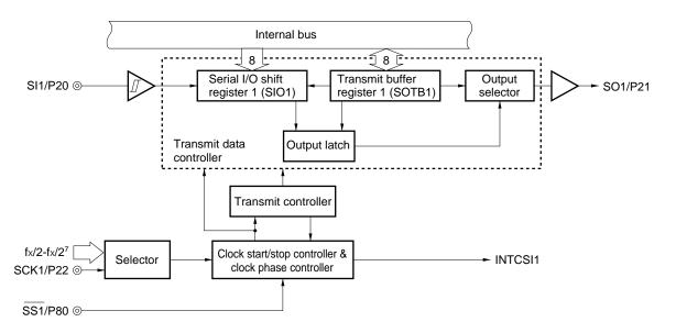
Figure 17-1. Serial Interface (CSI1) Block Diagram
