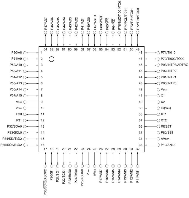
Cautions 1. Connect IC directly (Internally Connected) pin to Vsso or Vss1.
