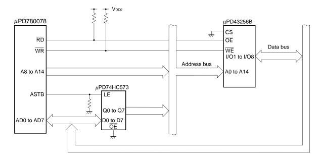
Figure 20-8. Connection Example of  $\mu$ PD780078 and Memory
