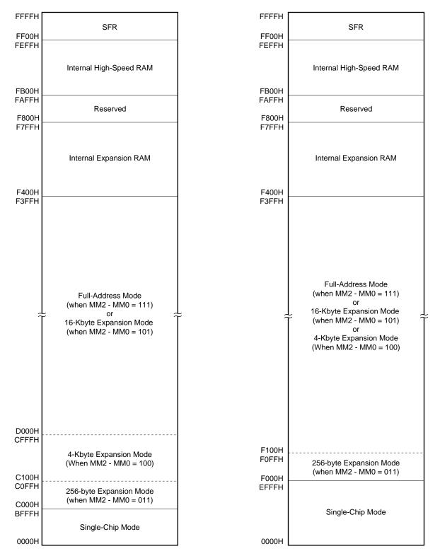
(b) Memory map of  $\mu$ PD780078, 780078Y and of  $\mu$ PD78F0078, 78F0078Y when flash memory size is 60 KB
