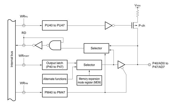
Figure 6-11. P40 to P47 Block Diagram
