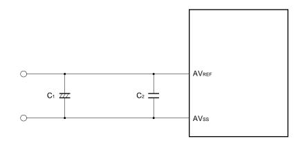
**Remark** C1: 4.7  $\mu$ F to 10  $\mu$ F (reference value) C2: 0.01  $\mu$ F to 0.1  $\mu$ F (reference value) Connect C2 as close to the pin as possible.
