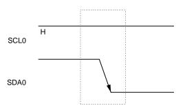
A start condition is output when the IIC control register 0 (IICC0)'s bit 1 (STT0) is set (to "1") after a stop condition has been detected (SPD0: Bit 0 = 1 in the IIC status register 0 (IICS0)). When a start condition is detected, IICS0's bit 1 (STD0) is set (to "1").
