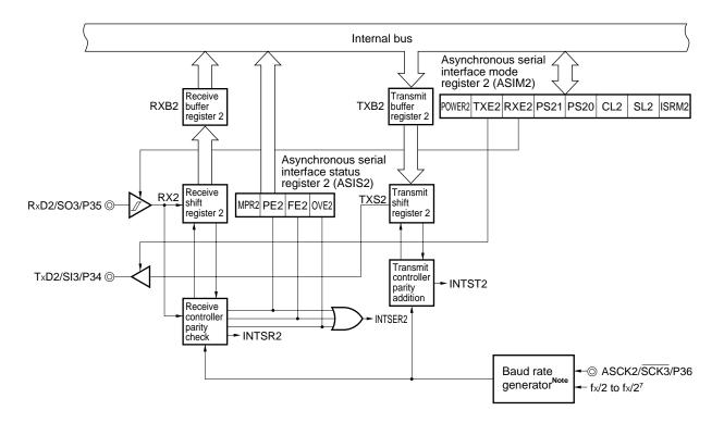
Figure 15-1. Serial Interface (UART2) Block Diagram
