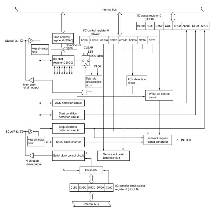
Figure 18-1. Serial Interface (IIC0) Block Diagram
