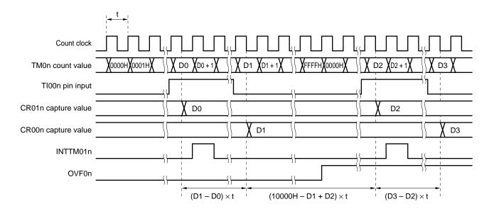
Figure 8-23. Timing of Pulse Width Measurement Operation by Free-Running Counter and Two Capture Registers (with Rising Edge Specified)
