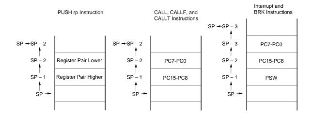
Figure 5-10. Data To Be Saved to Stack Memory
