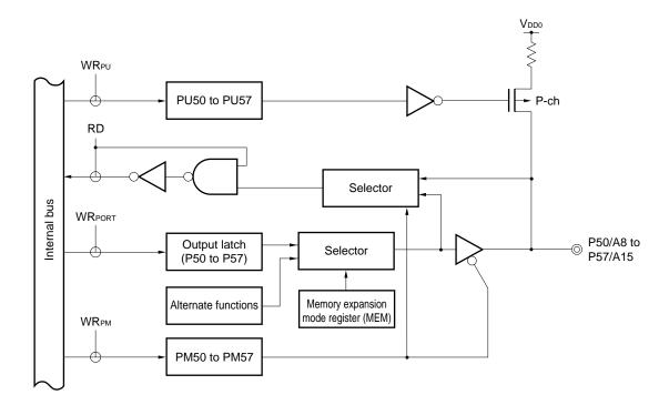
Figure 6-13. P50 to P57 Block Diagram
