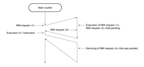
(b) If two non-maskable interrupt requests are generated during non-maskable interrupt servicing program execution
