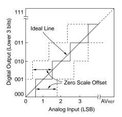
Figure 13-13. Integral Linearity Error
