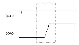
A stop condition is generated when bit 0 (SPT0) of the IIC control register 0 (IICC0) is set (to "1"). When the stop condition is detected, bit 0 (SPD0) of the IIC status register 0 (IICS0) is set (to "1") and INTIIC0 is generated when bit 4 (SPIE0) of IICC0 is set (to "1").
