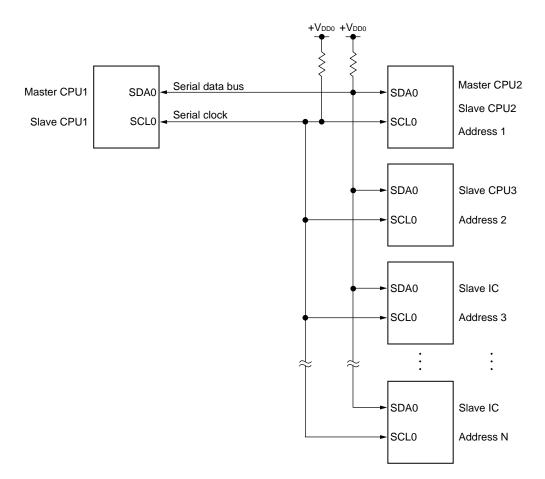
Figure 18-2. Serial Bus Configuration Example Using I<sup>2</sup>C Bus
