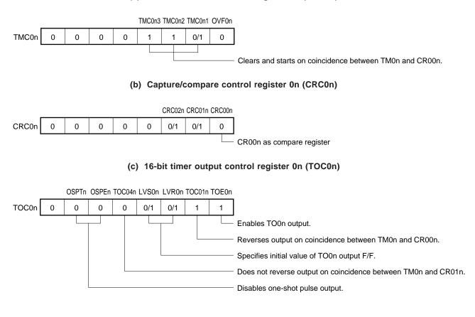
Remark 0/1: Setting 0 or 1 allows another function to be used simultaneously with square-wave output. See Figures 8-3 to 8-8.
