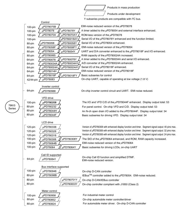
**Remark** VFD (Vacuum Fluorescent Display) is referred to as "FIP<sup>™</sup> (Fluorescent Indicator Panel) in some documents, but the functions of the two are the same.
