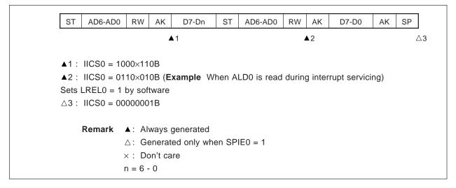
(e) When loss occurs due to stop condition during data transfer
