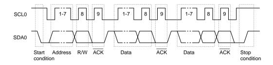
The master device outputs the start condition, slave address, and stop condition.
