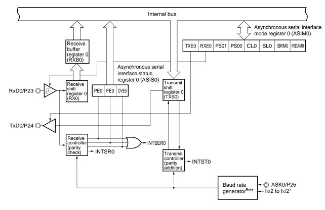
Figure 14-1. Serial Interface (UART0) Block Diagram
