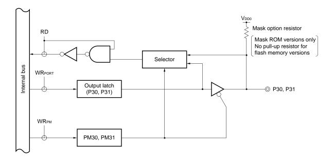
Figure 6-8. P30 and P31 Block Diagram (µPD780078Y Subseries)
