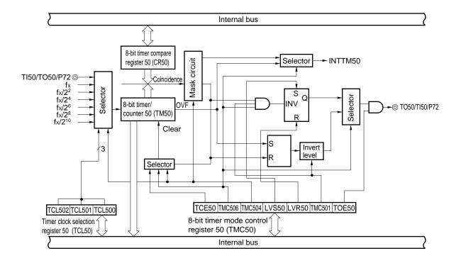
Figure 9-1. 8-Bit Timer/Event Counter 50 Block Diagram
