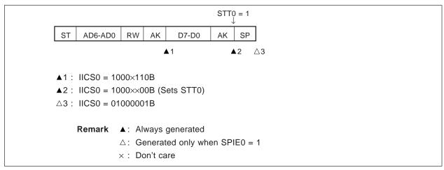
(h) When arbitration loss occurs due to low-level data when attempting to generate a stop condition
