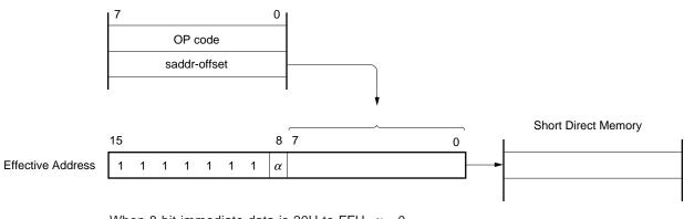
When 8-bit immediate data is 20H to FFH,  $\alpha = 0$ When 8-bit immediate data is 00H to 1FH,  $\alpha = 1$
