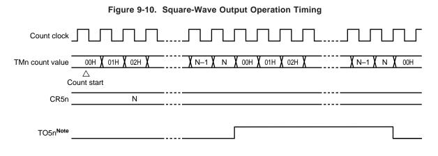
**Note** TO5n output initial value can be set by bits 2 and 3 (LVR5n, LVS5n) of the 8-bit timer mode control register 5n (TMC5n)
