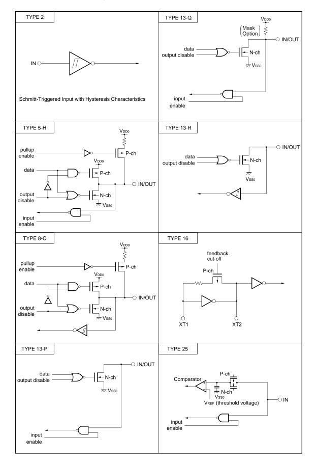
Figure 4-1. Pin Input/Output Circuit List
