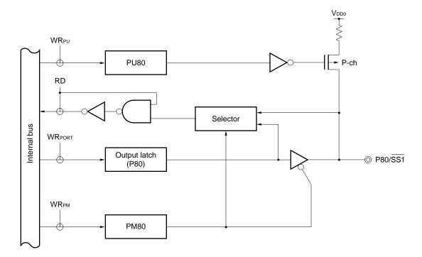
PU : Pull-up resistor option register
