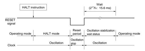
**Remarks 1.** fx: Main system clock oscillation frequency
