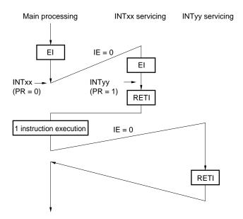
Interrupt request INTyy issued during servicing of interrupt INTxx is not acknowledged because its priority is lower than that of INTxx, and nesting does not take place. The INTyy interrupt request is held pending, and is acknowledged following execution of one main processing instruction.
