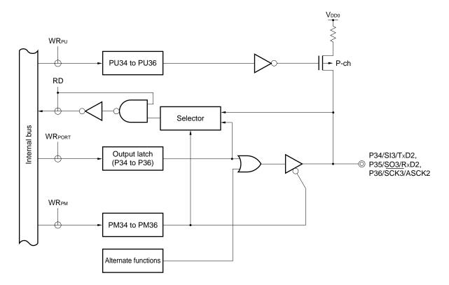
Figure 6-7. P34 to P36 Block Diagram (µPD780078 Subseries)
