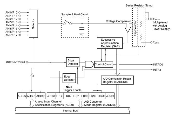
Figure 13-1. 10-Bit A/D Converter Block Diagram
