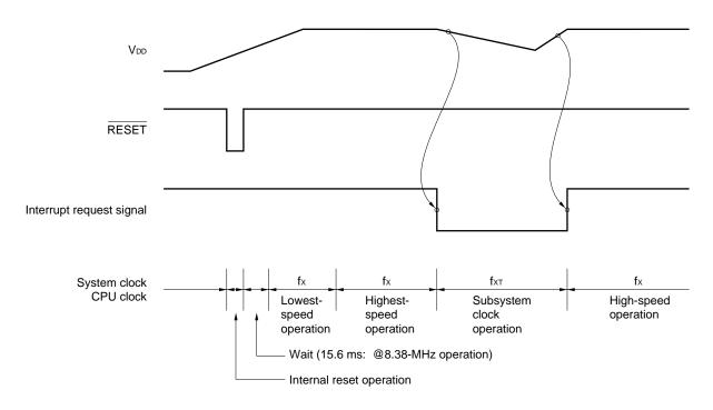
Figure 7-8. System Clock and CPU Clock Switching
