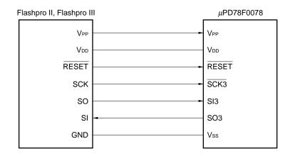
Figure 23-4. Connection of Flashpro II and Flashpro III Using 3-Wire Serial I/O (SIO3) Method
