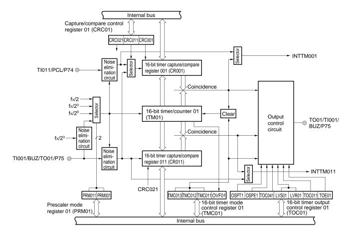
Figure 8-2. 16-Bit Timer/Event Counter 01 Block Diagram
