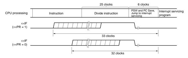
Figure 19-12. Interrupt Request Acknowledge Timing (Maximum Time)
