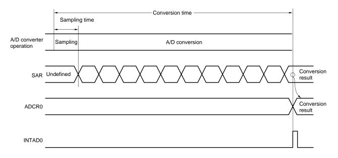
A/D conversion operations are performed continuously until bit 7 (ADCS0) of the A/D converter mode register 0 (ADM0) is reset (0) by software.
