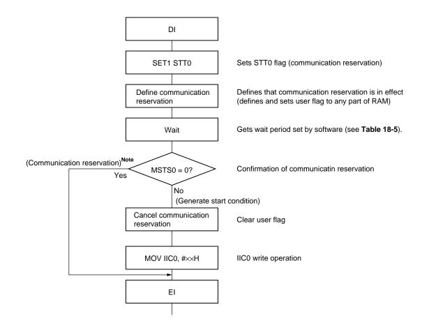
**Note** The communication reservation operation executes a write to the IIC shift register 0 (IIC0) when a stop condition interrupt request occurs.
