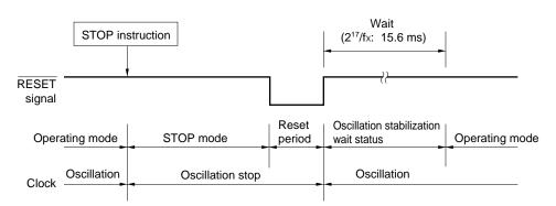
Figure 21-5. STOP Mode Release by RESET Input
